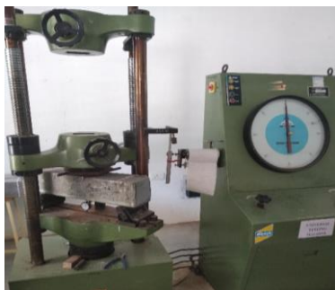
Figure 10: Wrapped Beam Setup
