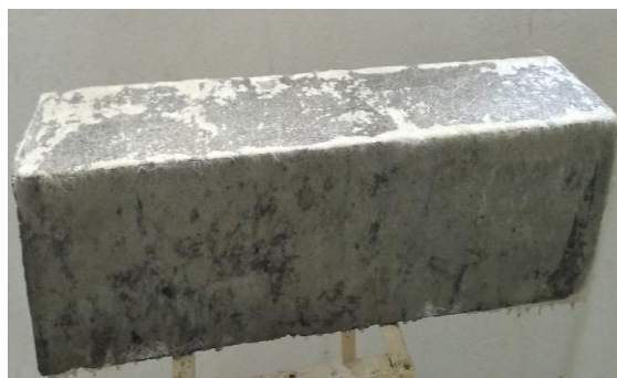
Figure 11: E-glass Wrapped Beam
