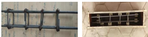
Figure 1: Reinforcement and mould setup
