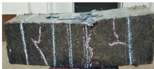
Figure 14: Failure pattern of basalt fiber wrapped beam
